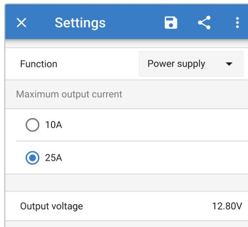
It is also possible to enable low current mode while in power supply mode and to specify the desired output voltage.
